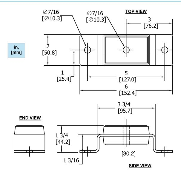
CRM Mounts allow the use of any bolt type fasteners or threaded rod up to 3/8" dia. (10mm) in any length to suit application. The use of nylon insert self locking type nut is recommended.
