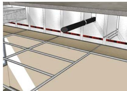
Secure the 3 tape edges of the RAS (closed end & 2 long sides) to the Privacy Board™ with FSK tape supplied.
