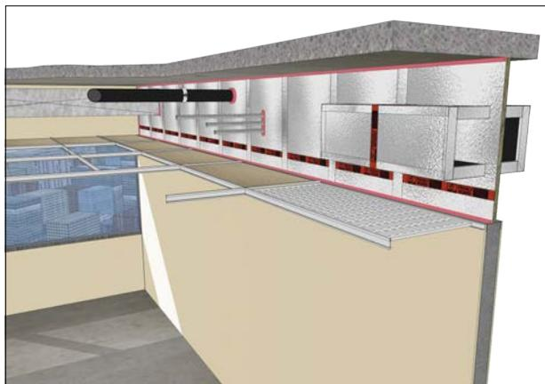
View from above a suspended ceiling showing a complete Privacy Board™ installation with Return-Air Silencers
